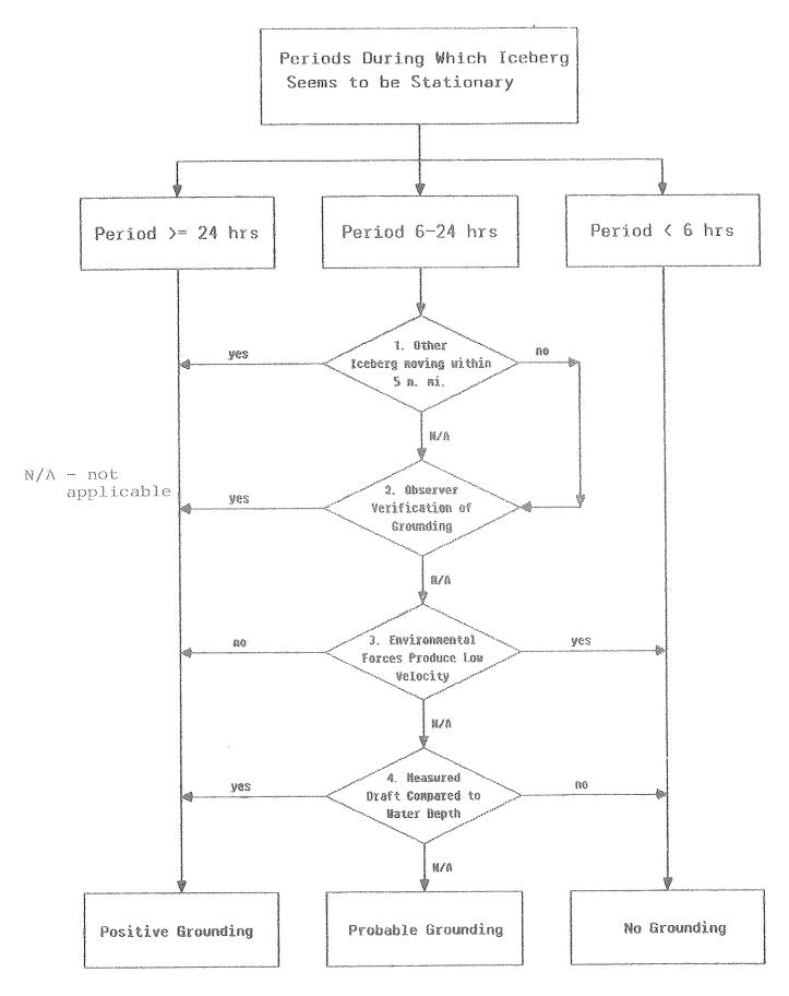
Fig. 1 Grounding Criteria for Iceberg Tracked by Drill-Rig or Shore-Based Radar
