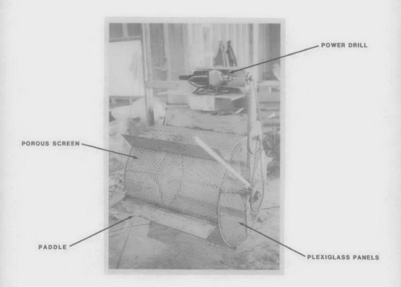
The drum apparatus was suspended from the same cart as used for the porous plane; the support connections could be varied to change the submergence of the drum. Drive for the drum rotation was provided by a variable speed drill with a chain and gear arrangement with 30:1 gear reduction.
