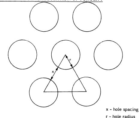
Holes punched in the pattern of a series of equilateral triangles.
