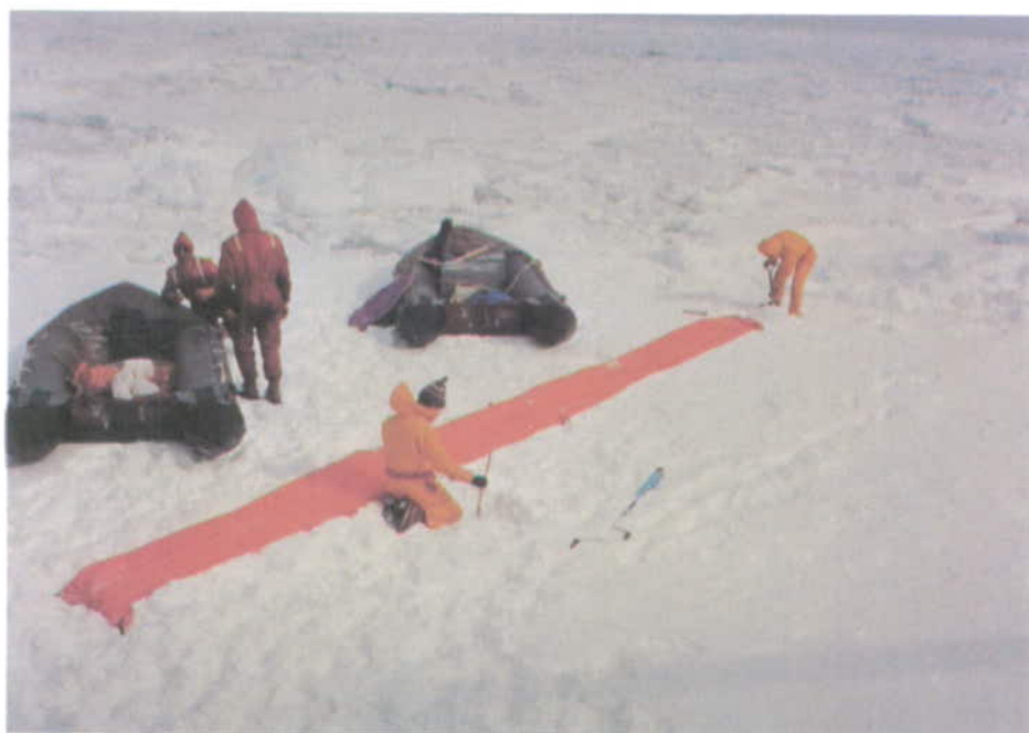
Figure 12 - Coloured nylon strip for aerial photo scale
