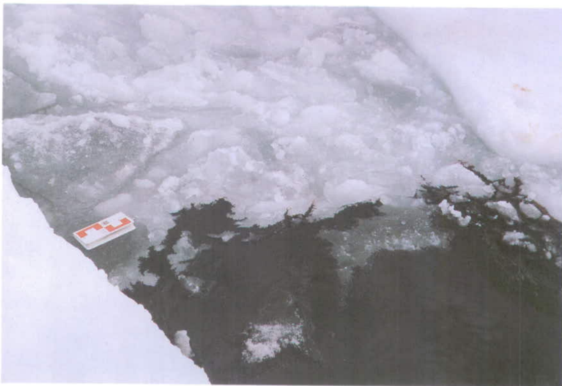
Figure 41 - Oil on top of slush and brash ice between the two floes in the lower left and upper right corners of the photograph. Picture taken within 20 min of oil release
