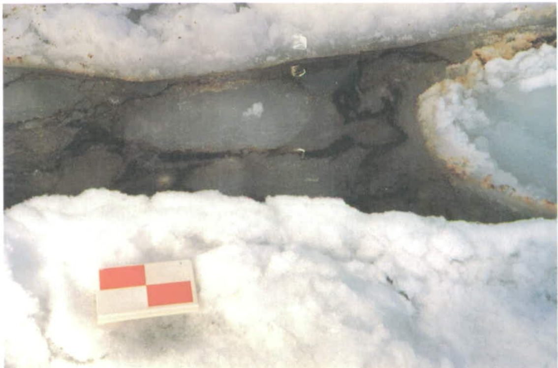
Figure 37 - Close-up view of oiled slush and brash ice being squeezed between two first-year floes. Part of an ice pancake is visible to the right.
