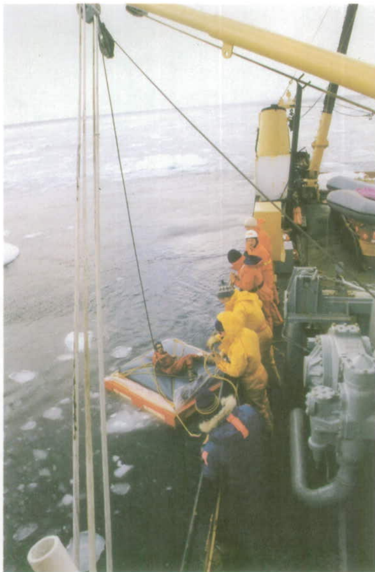
Figure 6 - Placement of spill raft
