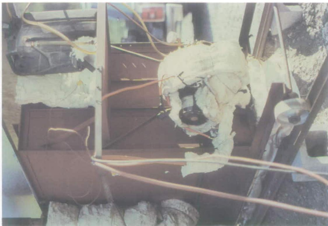
Photo No.3 - The burner end of the combustion box showing the oxygen hose connection.
