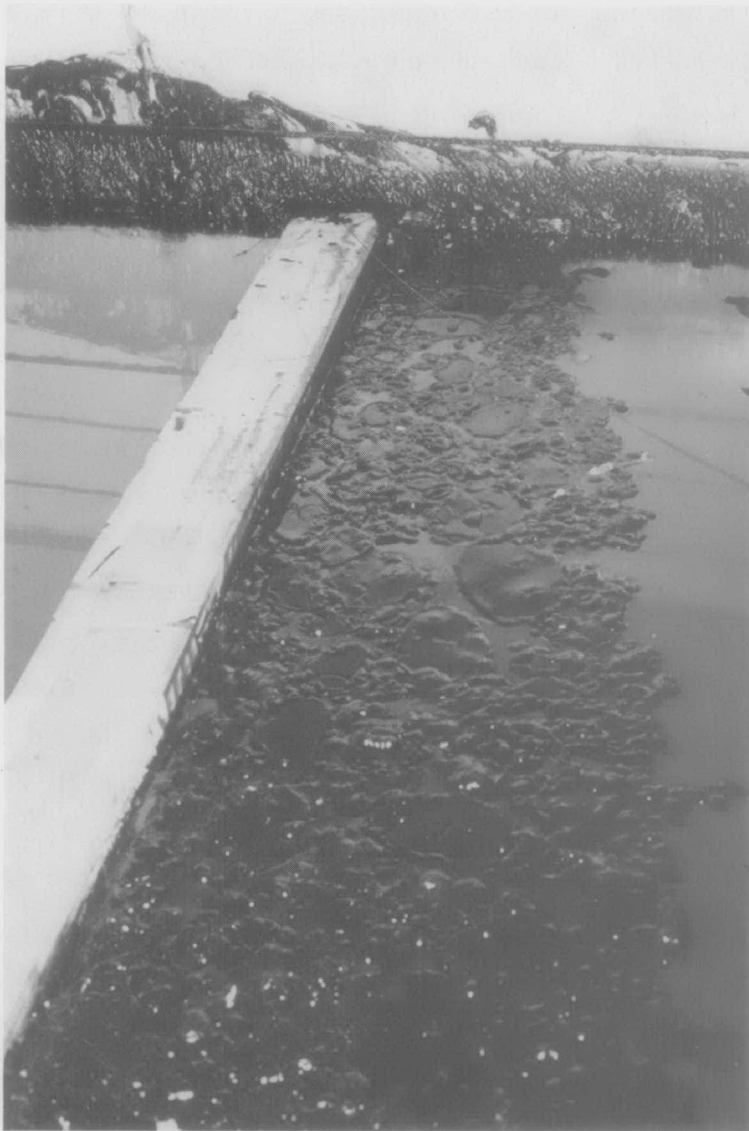
Figure 45: Consolidation of oil patches against boom (run B7)
