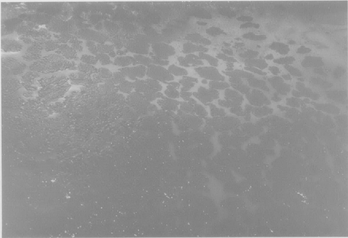
Figure 46: Agglomeration of oil droplets, five minutes after discharge (run B10)
