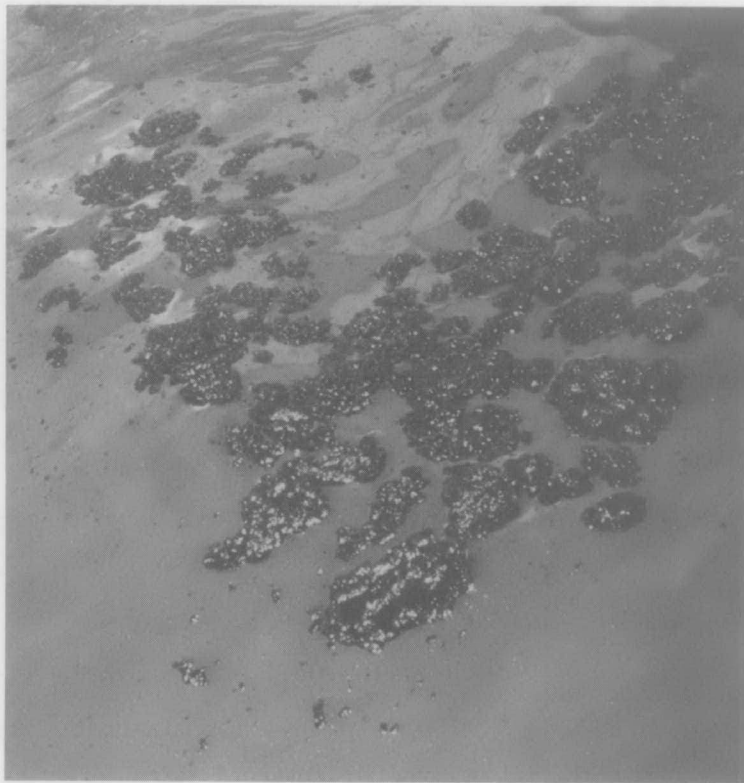
Figure 50: Clumping of matted oil droplets, 15 minutes after discharge (run B17)
