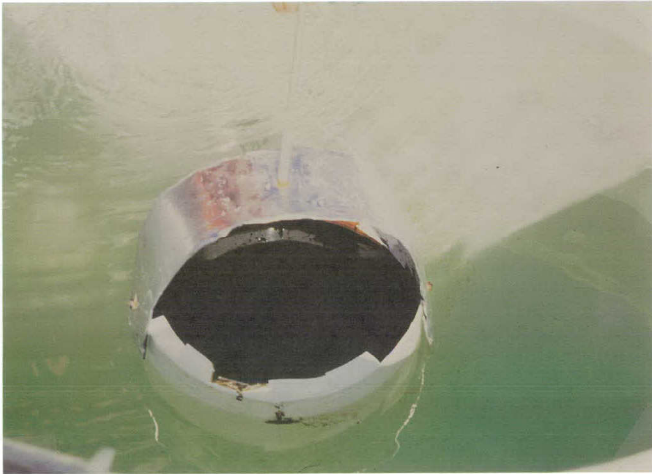
FIGURE 4. Containment ring positioned on the water surface at the centre of the simulator.
