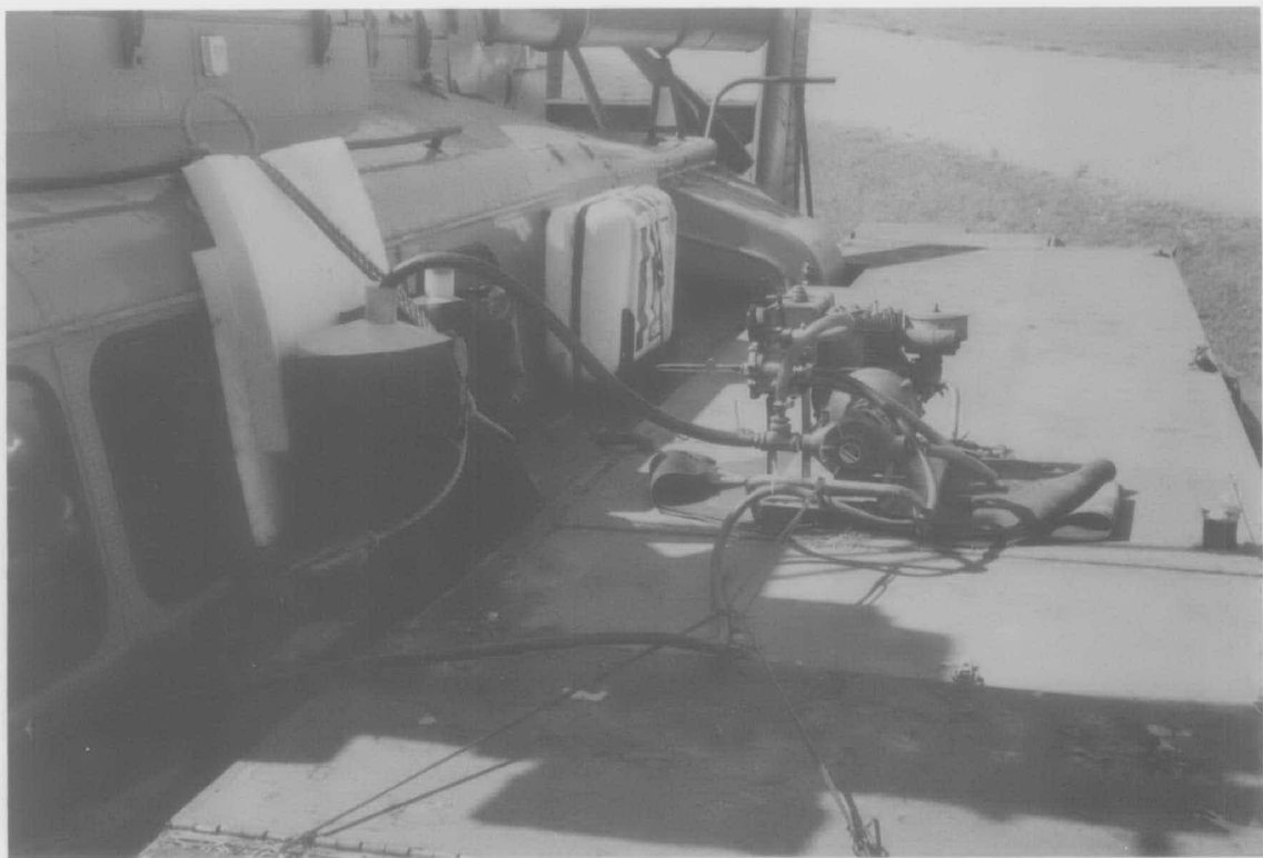
Figure 12. Dispersant tanks and spray pump
