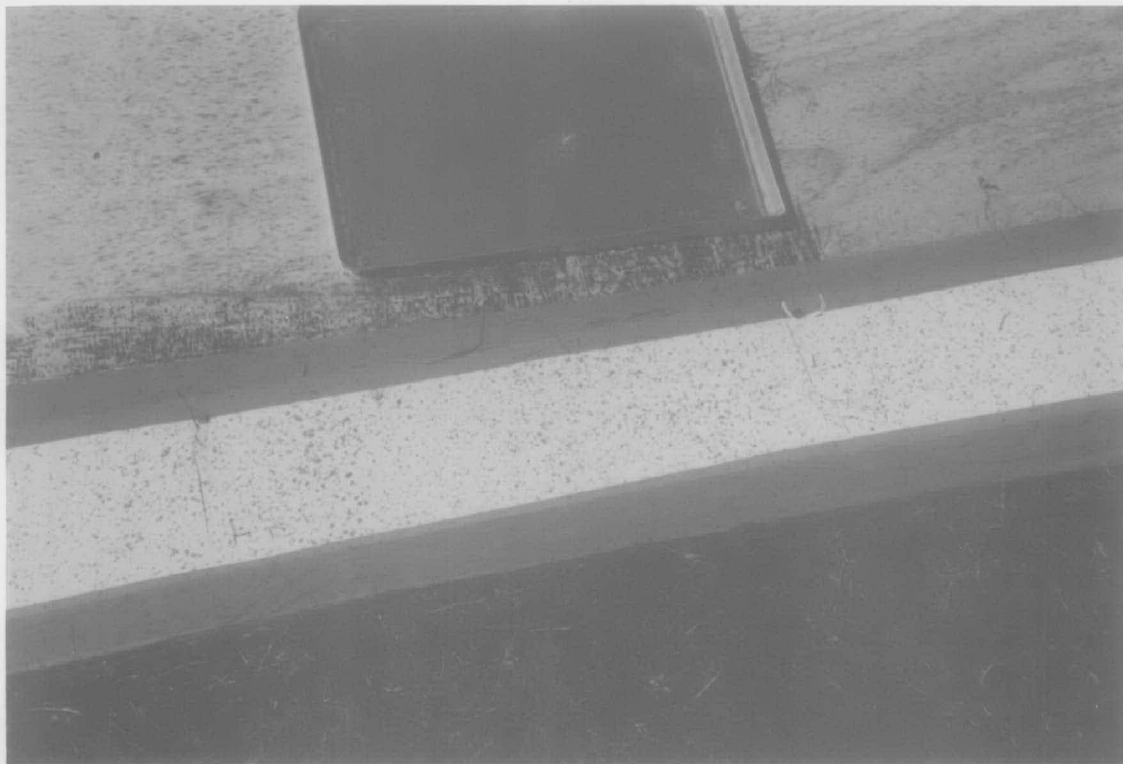
Figure 21. Example dispersant spray pattern
