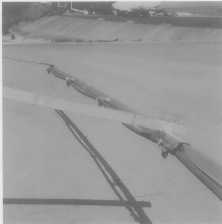
Figure 11. Close-up view of dispersant spray boom
