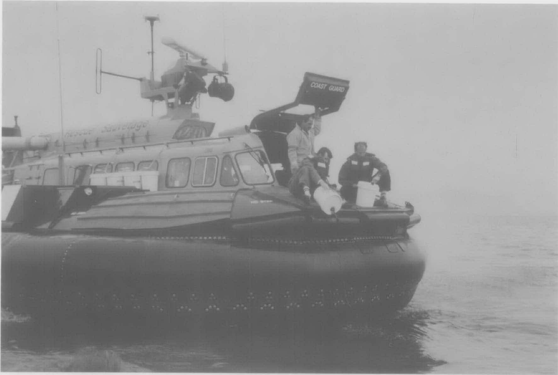
Figure 4. Canola oil being discharged off the bow of the hovercraft
