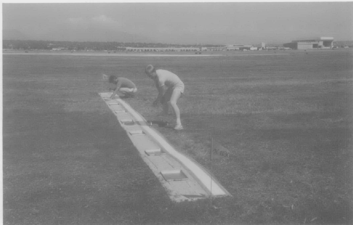
Figure 14. Laying out the Kromekote cards and collection trays across the hovercraft course
