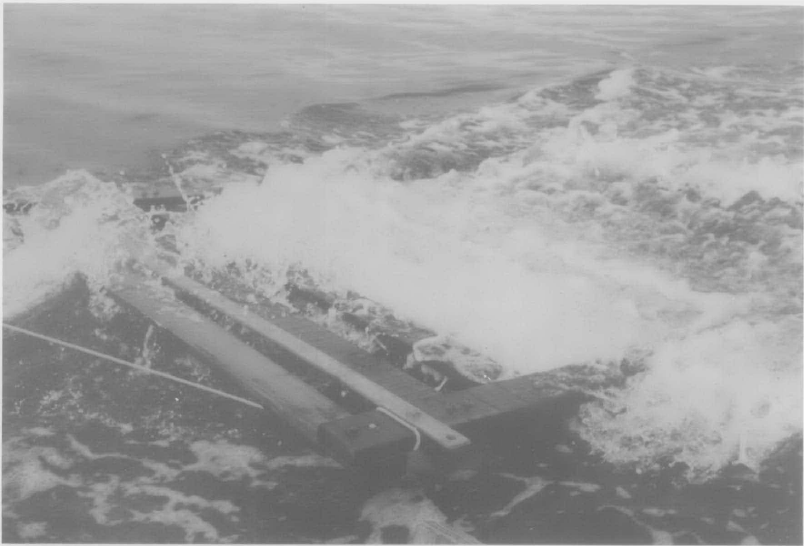
Figure 7. Breaker board being towed through dye cloud
