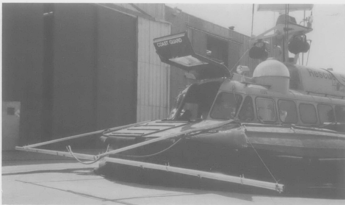
Figure 10. General view of dispersant spray boom
