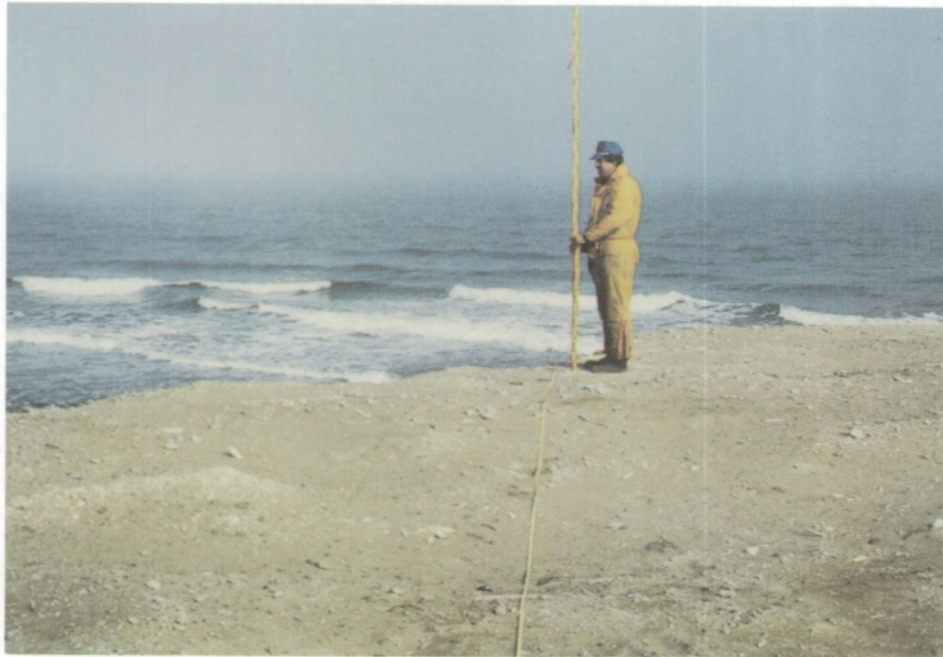
Figure 3.2 Surveying island surface with tape and rod along line 000 as viewed due north. Waves are breaking on the wing bar on the northwest corner of the island. (August 10, 1986).
