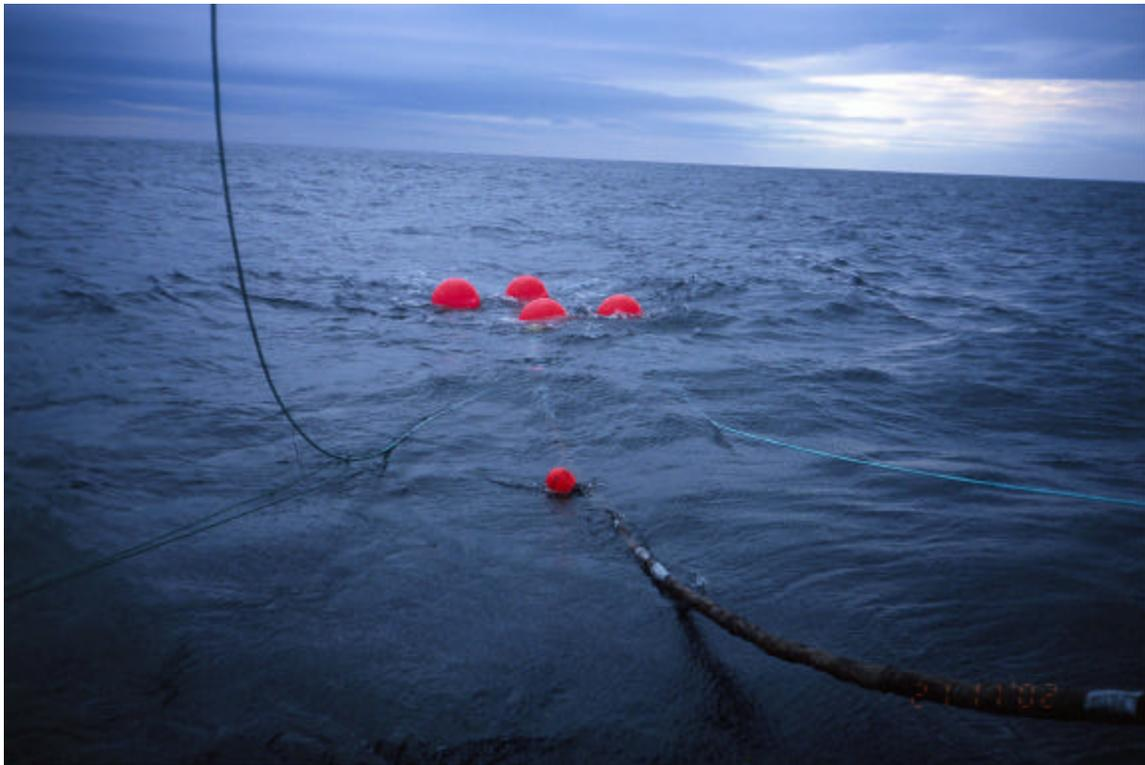
Figure 7. 200-in<sup>3</sup> array firing off the stern of *FV Rough and Wild*.
