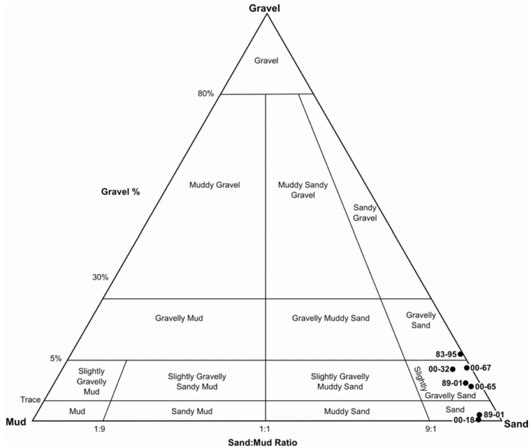
Figure 20: Gravel, sand and mud diagram of grain size analyses from the IKU grab samples.
