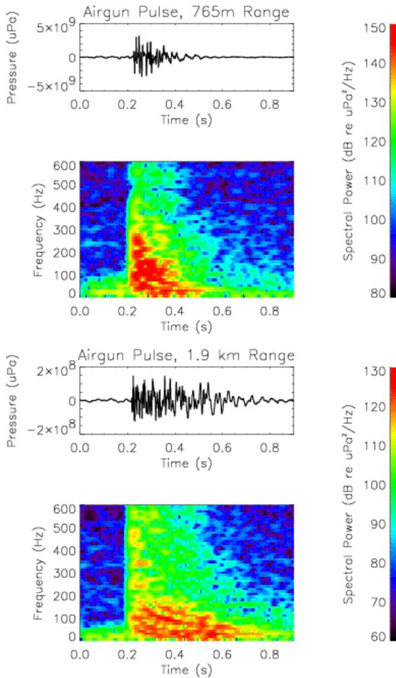
**Figure 1.8: Plots of the pressure and spectral power for an individual airgun pulse measured on Dec. 20, 2003 at 1900-m range (right) and 765-m range (left). Admiral was acquiring data along line CHT-109-09 during these measurements.**
