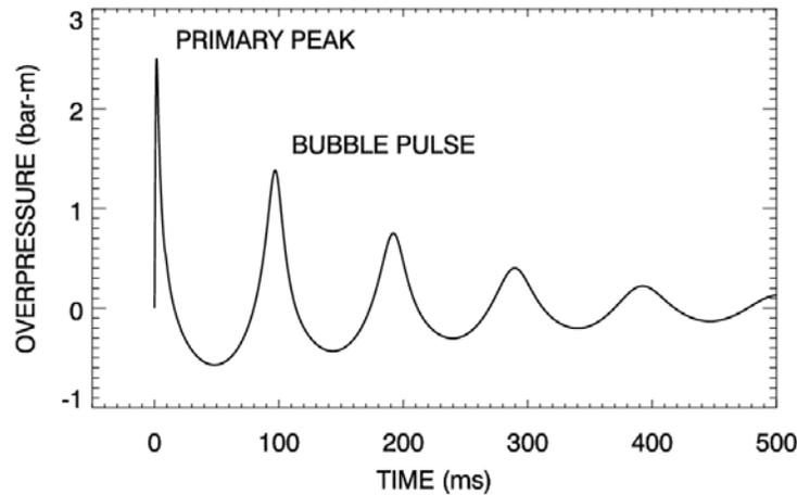
**Figure 1.1: Overpressure signature for a single airgun, showing the primary peak and the bubble pulse.**
