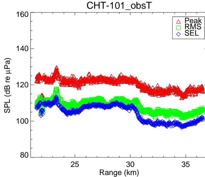
**Figure 1.12: Peak, RMS, and sound exposure level measurements versus range obtained at OBS-T at 85-m depth at the control site. Measurements were taken during seismic Line CHT-101-01 with a heading of 89 degrees on the closest approach to the control site on Dec. 15, 2003.**
