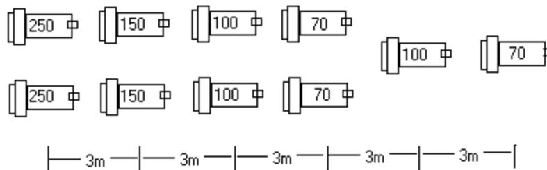
**Figure 1.4: Airgun array layout.**
