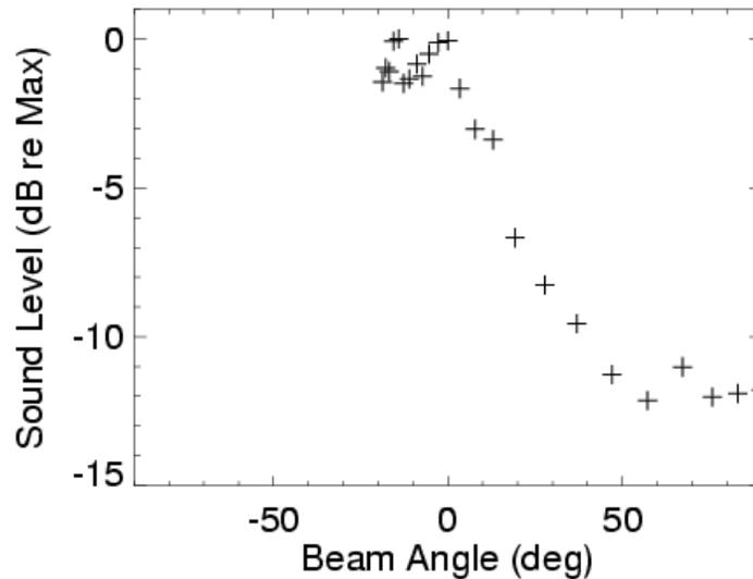
**Figure 1.6: Airgun array directivity pattern. Sound levels are normalized to the maximum broadside levels (i.e., sound levels are 0 dB at the broadside peak) and corrected for spherical spreading loss.**
