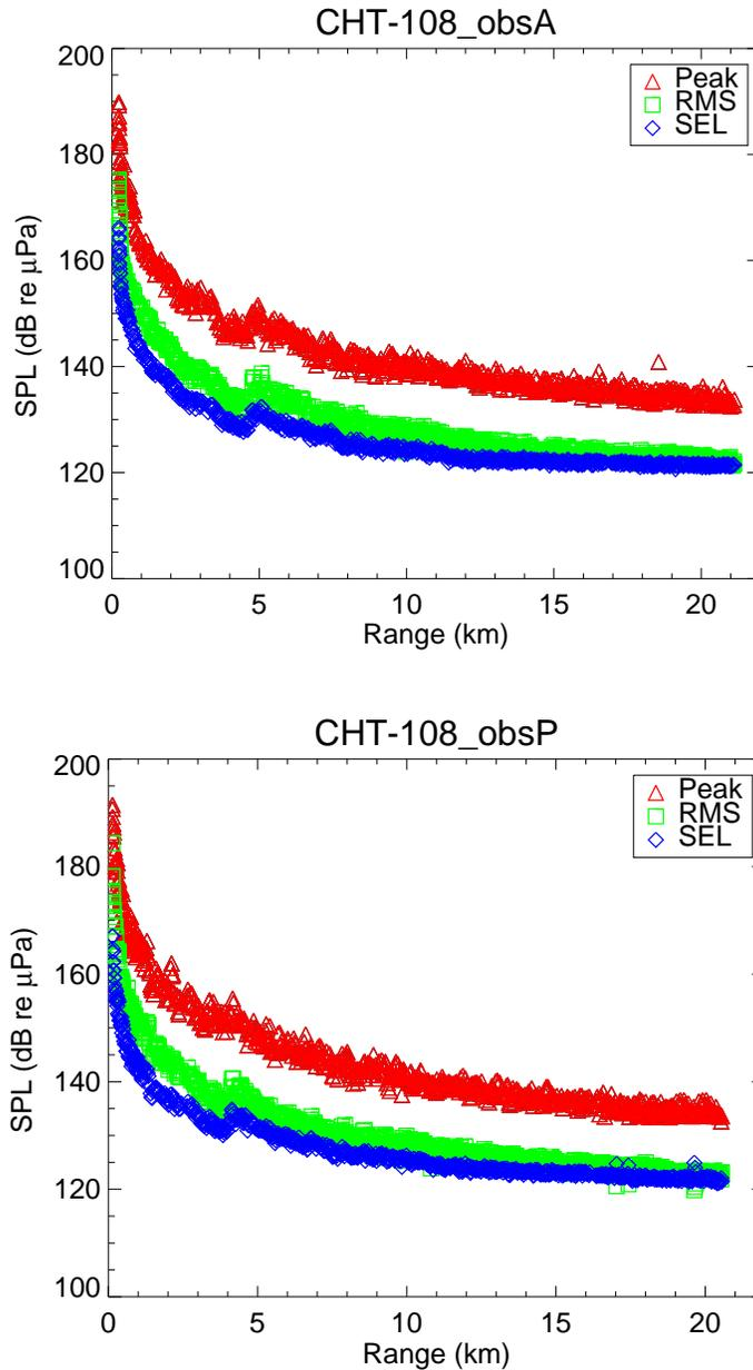
**Figure 1.9: Peak, RMS, and sound exposure level measurements versus range obtained at OBS-A at 63-m depth (top panels) and OBS-P at 70- m depth (bottom panels) at the crab test site. Measurements were taken during seismic Line CHT-108-08 with a heading of 269 degrees through the test site on Dec. 20, 2003.**
