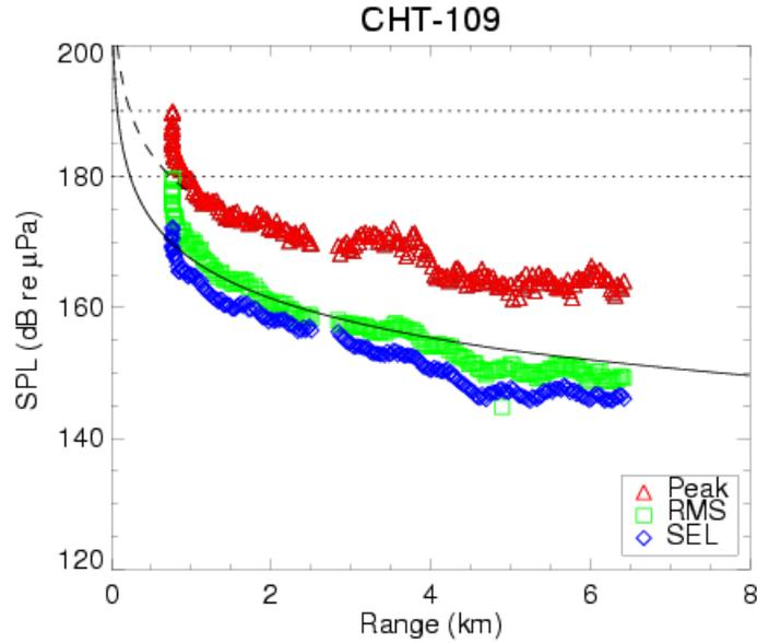
**Figure 1.7: Peak, RMS, and sound exposure level measurements versus range at 34-m depth during seismic Line CHT-109-09 on Dec. 20, 2003. Solid black line indicates a fit of the transmission loss equations to the data beyond 1-km range (“endfire” levels). Dotted black line indicates a fit of the transmission loss equations to the data within 1 km range (“broadside” levels).**
