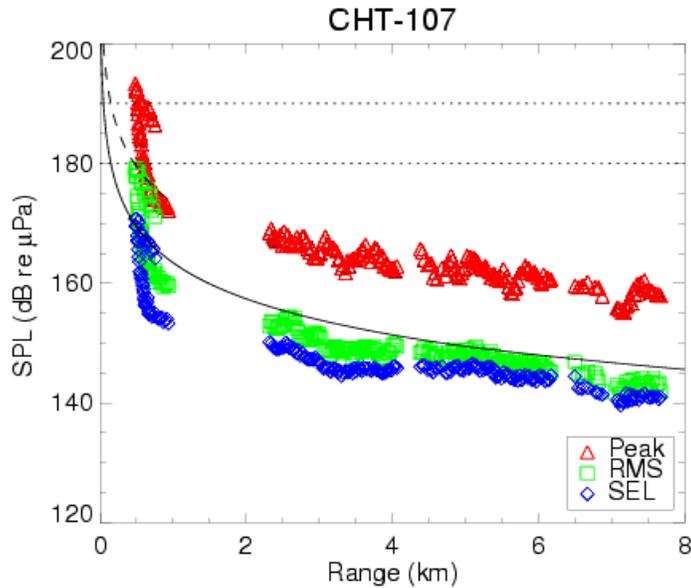
**Figure 1.5: Peak, RMS, and SEL measurements as a functions of range at 34-m depth during seismic Line CHT-107-07 on Dec. 20, 2003. Solid black line indicates a fit of the Marsh and Schulkin transmission loss equations to the RMS data beyond 1 km range (“endfire” levels). Dotted black line indicates a fit of the Marsh and Schulkin transmission loss equations to the RMS data within 1 km range (“broadside” levels).**
