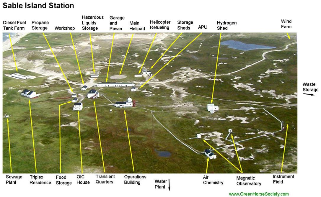
**Figure 2:** Overview of Sable Island Station Showing the Location of Various Buildings and Associated Equipment. The air monitoring equipment is located in the air chemistry building on the bottom right of the diagram. The view is looking east-southeast. *(Courtesy of Zoe Lucas)*
