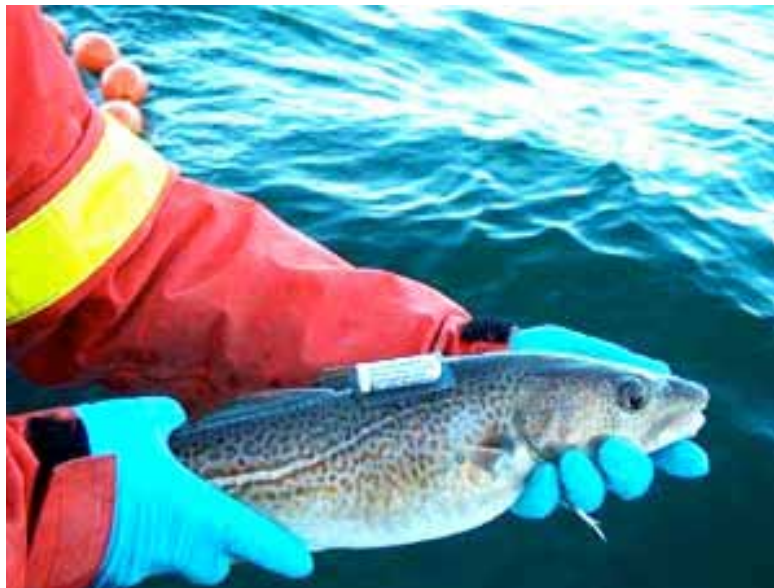
Figure 10. An archival (data storage) tag attached to a cod. Image from Star-Oddi website
