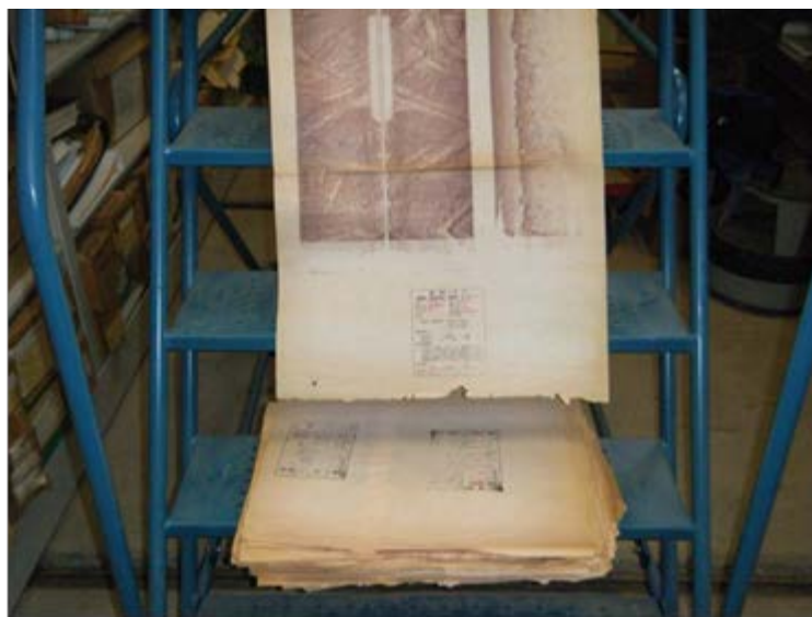
Fig. 7. Side-scan sonar records on folded wet paper. These sonar records were well-marked with the stamps indicating where and when the data were collected.
