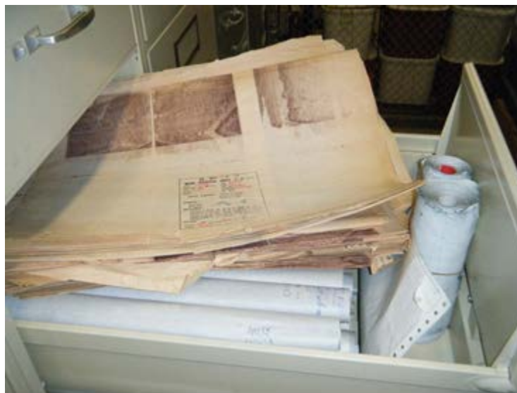
Fig. 5. Drawer with seismic, sonar, and bathymetry data. The long seismic rolls are lying flat; the smaller, thicker bathymetry rolls are upright at the front of the drawer. Sonar records are on folded wet paper and generally stamped with time and location information.
