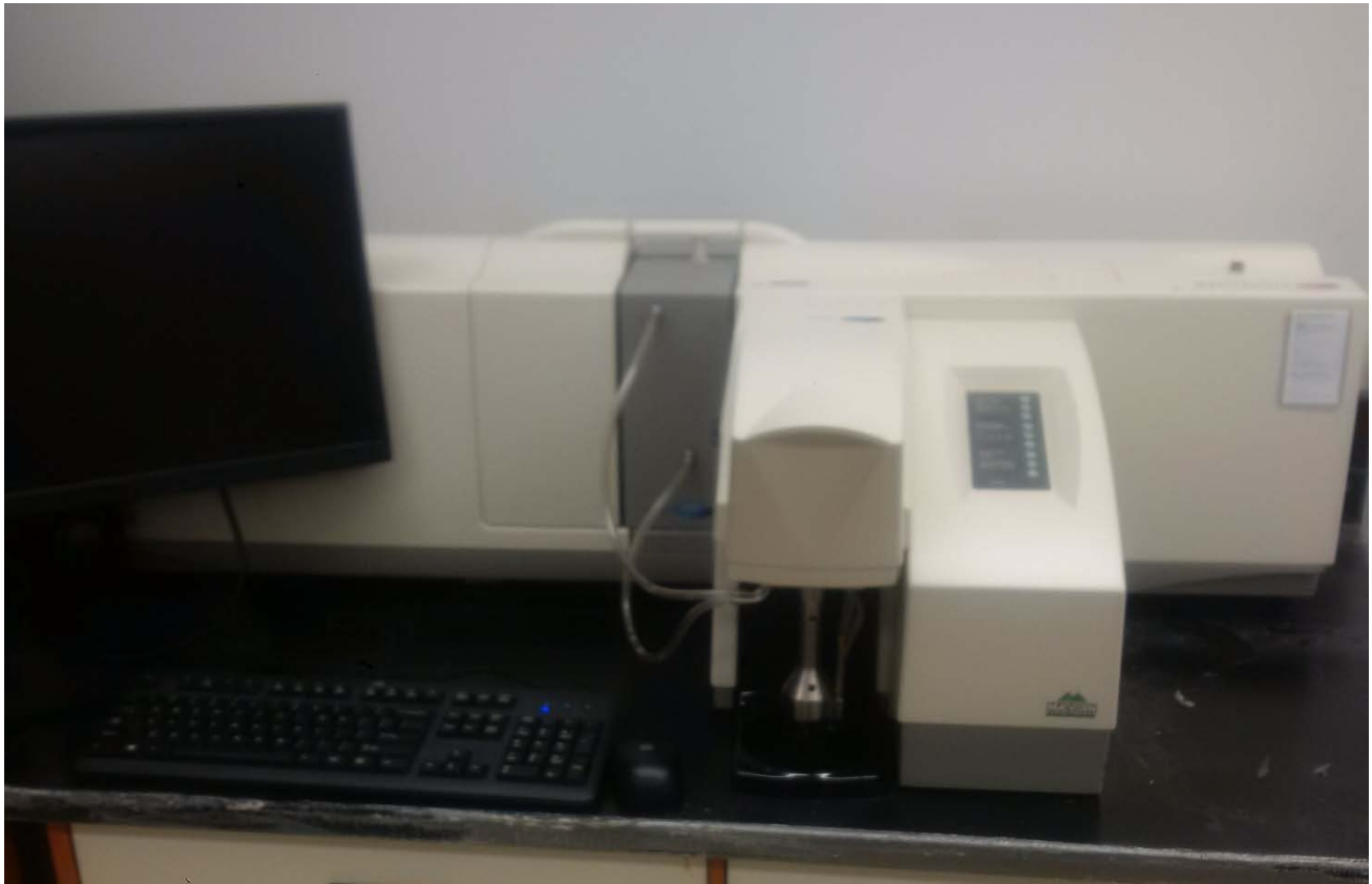
Figure 9. A picture of the ESTS's Malvern Mastersizer 2000 particle size analyser with the Hydro 2000 Unit used to measure grain size distribution of the selected sediment samples.
