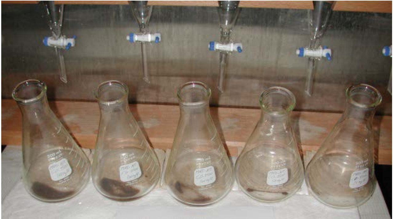
Figure 24. Remaining oil-sediment mixture (negatively buoyant OSAs) after careful elimination of the floating materials and water. Samples shown are ready for transfer into separatory funnels. Note the sediment concentration used in this experiment increases from right to left.
