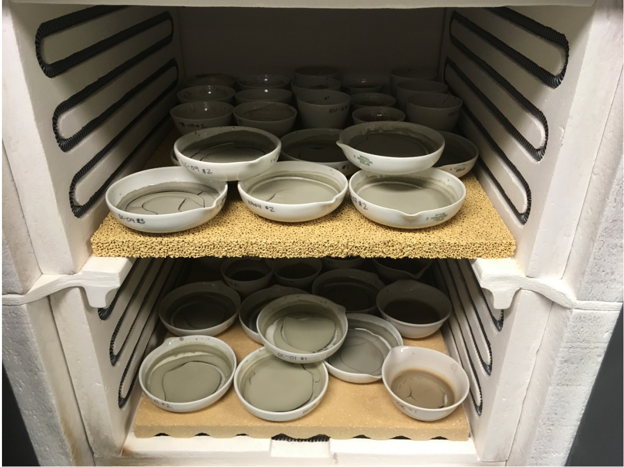
Figure 8. A picture of the crucibles containing sediment samples when introduced into the furnace during the Loss-on-Ignition experiment to measure organic matter content in the sediments.
