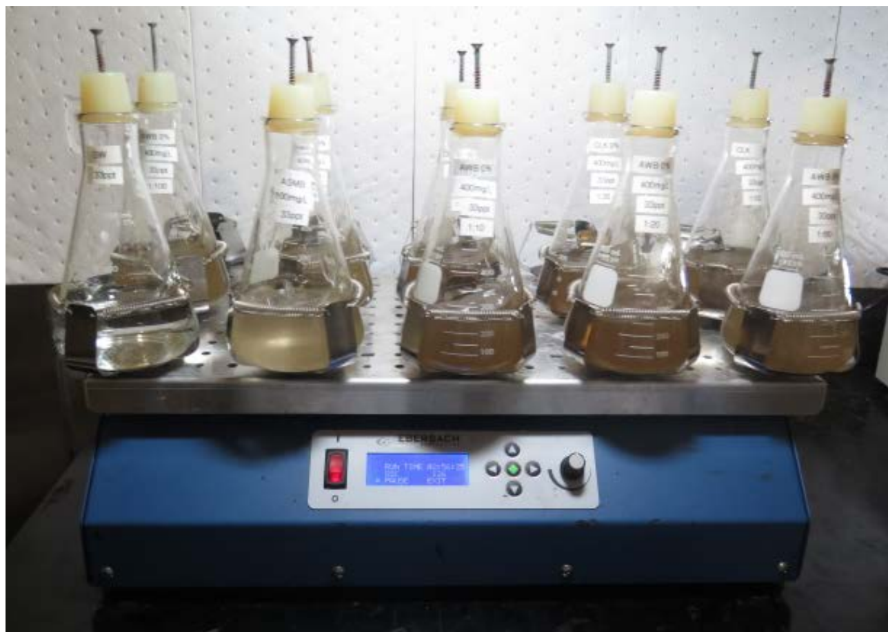
Figure 23. Reaction vessels set for shaking on the reciprocating shaker
