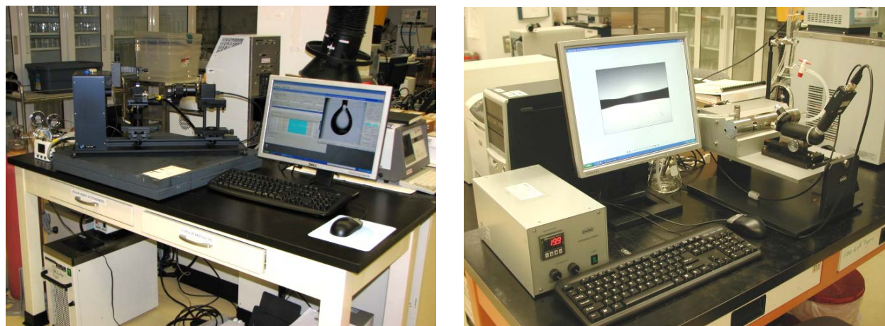
Figure 11. Instruments used to measure oil/brine interfacial tension: KSV CAM200 Pendant Drop (left), and KRUSS spinning Drop SITE100 (right).
