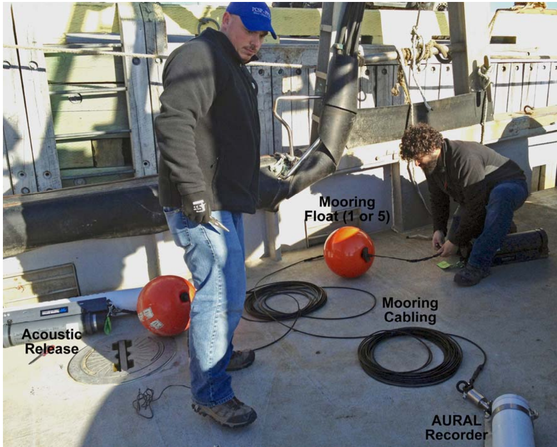
Figure 29. Assembling the mooring systems for AURAL acoustic recorders.
