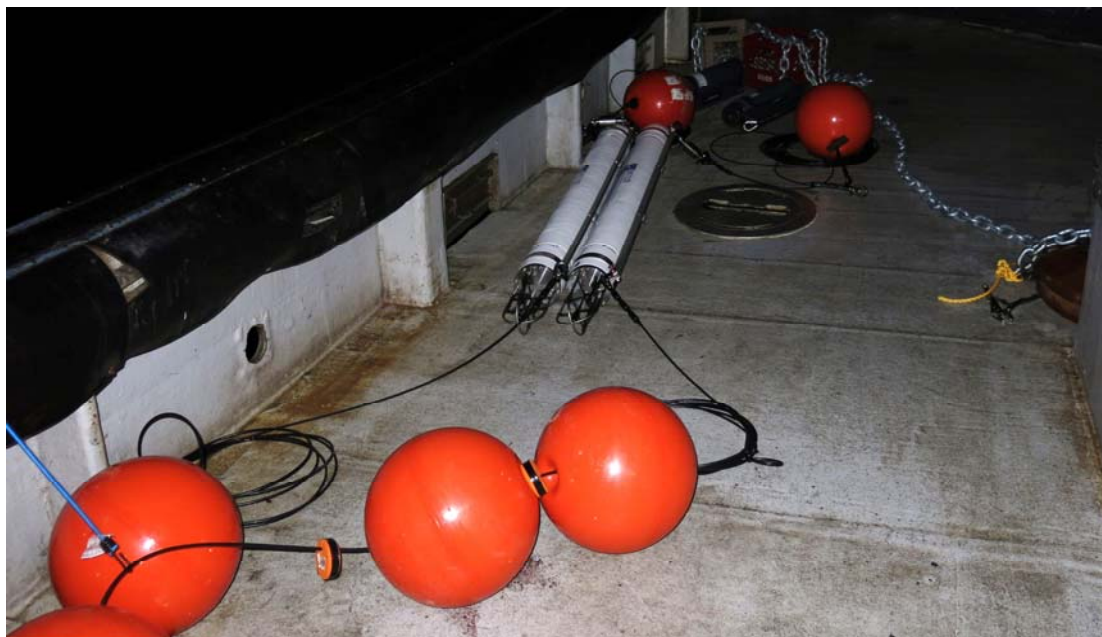
Figure 30. Mooring systems for two AURAL recorders (white cylinders) prepared and en route for deployment in the study area in October 2013.
