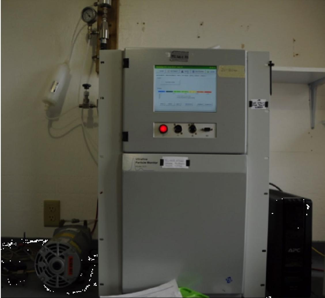
**Figure 16 TSI Ultrafine Particle Monitor (UFPM) model 3031**
