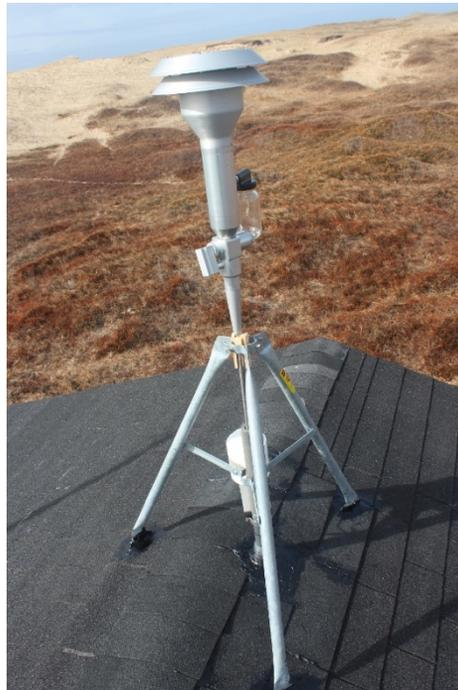
**Figure 9 Sampling inlet for the Thermo Scientific 5012**
