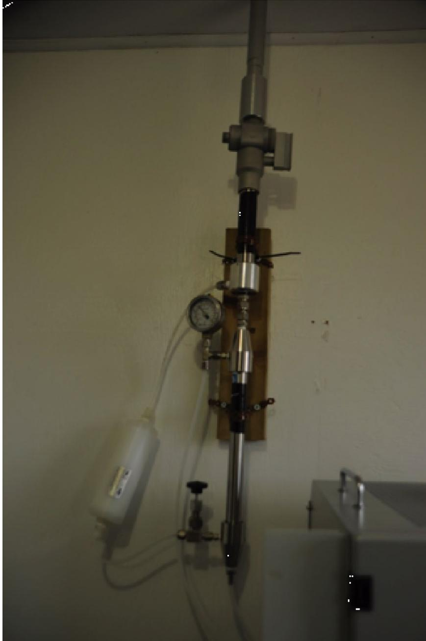
**Figure 17 TSI 3031200 Environmental Sampling System (ESS)**
