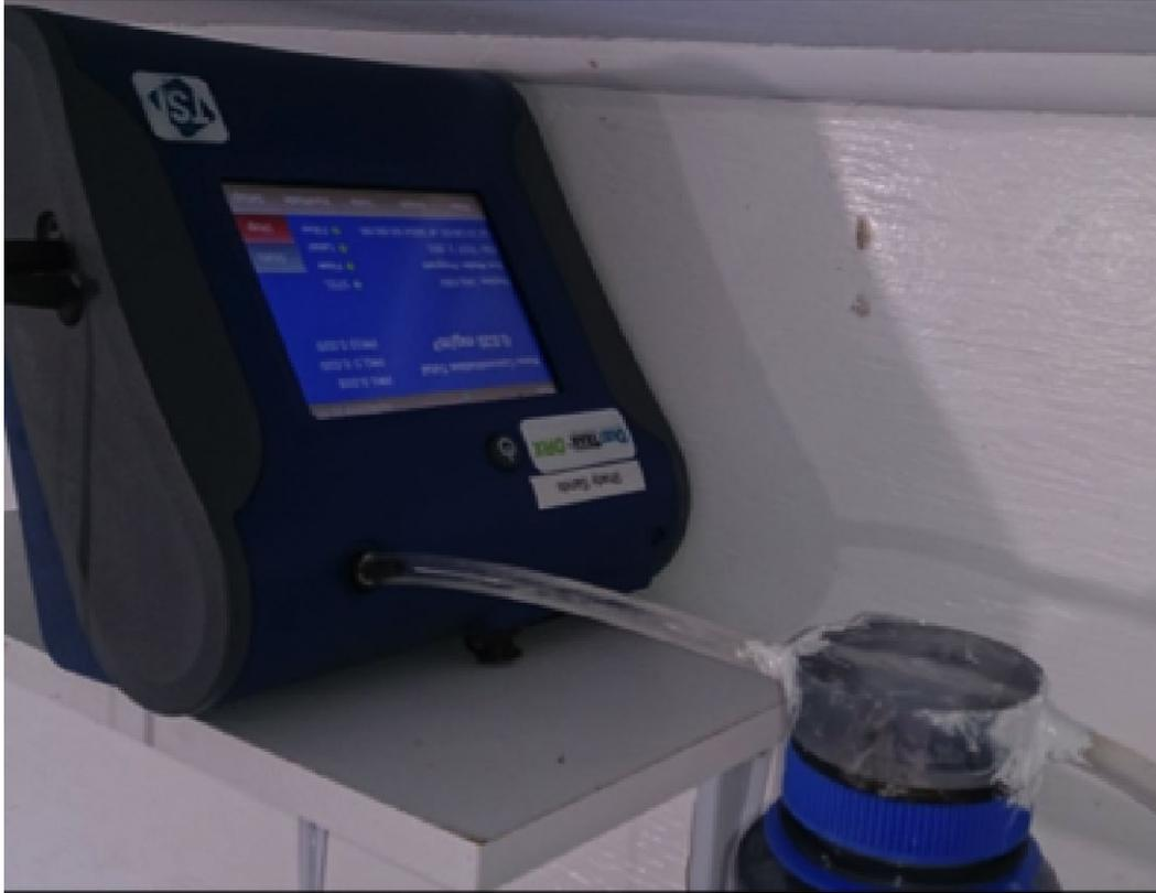
**Figure 14 TSI DustTrak DRX Aerosol Monitor model 8533 (Photo Courtesy of Codey Barnett)**
