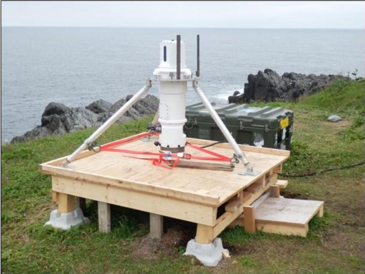
FIGURE 6. The FIRSTnavy sensor was situated on a level platform near the cliff edge at Cape Race, NL.
